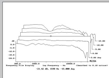
**Fig.5** Göbel Divin Marquis, vertical response family at 1m, normalized to response on tweeter axis, from back to front: differences in response 15-5° above axis, reference response, differences in response 5-10° below axis.
