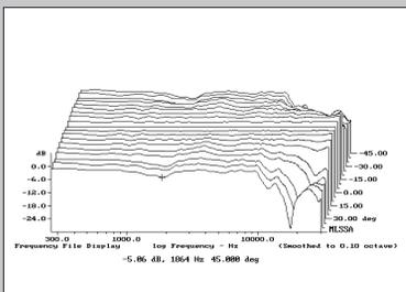
**Fig.4** Göbel Divin Marquis, lateral response family at 1m, normalized to response on tweeter axis, from back to front: differences in response 45-5° off axis, reference response, differences in response 5-45° off axis.
