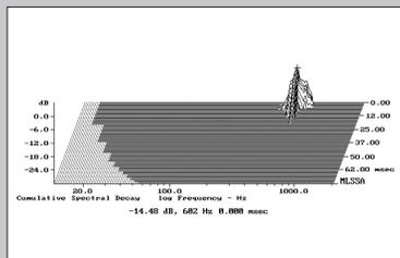
Fig.2 Göbel Divin Marquis, cumulative spectral-decay plot calculated from output of accelerometer fastened to center of top panel close to rear (MLS driving voltage to speaker, 7.55V; measurement bandwidth, 2kHz).
