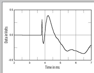
**Fig.8** Göbel Divin Marquis, step response on tweeter axis at 50" (5ms time window, 30kHz bandwidth).
