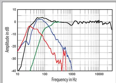
Fig.3 Göbel Divin Marquis, anechoic response on tweeter axis at 1m, averaged across a 30° horizontal window and corrected for microphone response with the nearfield responses of the midrange unit (green), woofer (blue), and ports (red), respectively plotted below 300Hz, 1kHz, and 600Hz.
