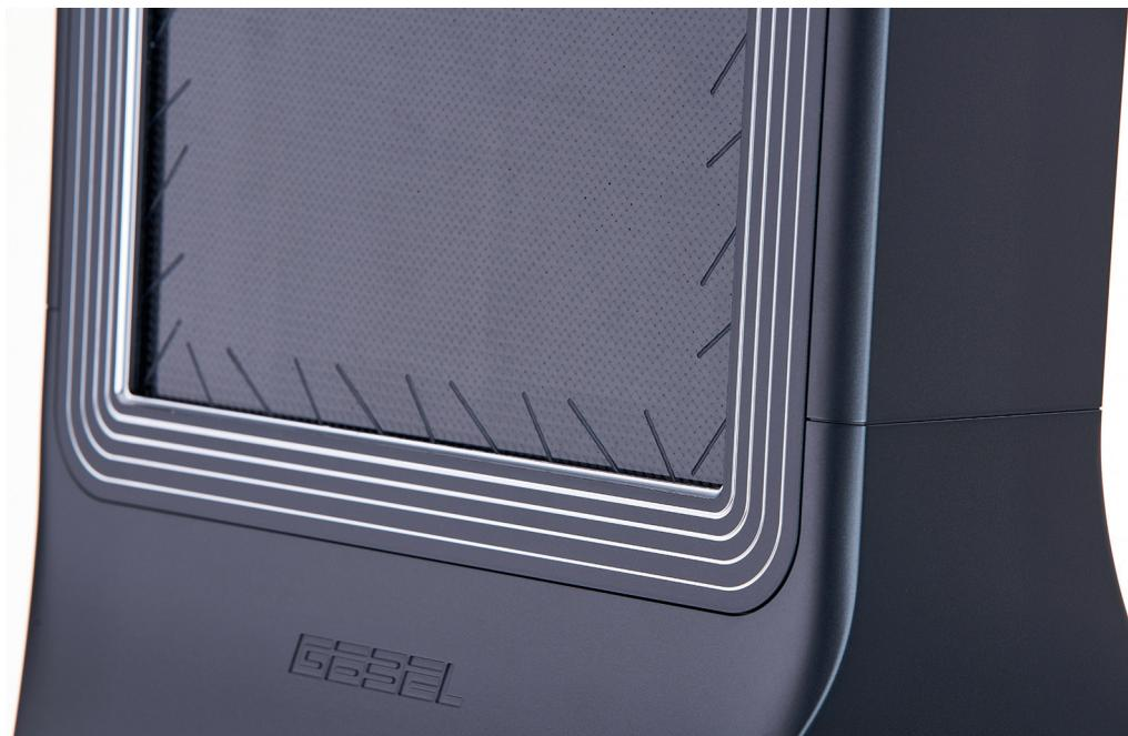
*The incisions in the nine-layer membrane are intended to diffusely dissipate parasitic oscillation energies so that standing wave fields are avoided to emerge. The angles and positions of the incisions are calculated exactly to a hundredth of a millimeter and are cut by a laser*
