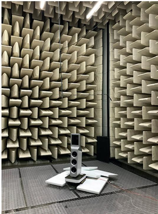
*The Epoque Aeon Fine in the anechoic measuring room of the Technical University of Deggendorf, Bavaria, where even frequencies of 40 Hertz are still absorbed to 99 percent*
